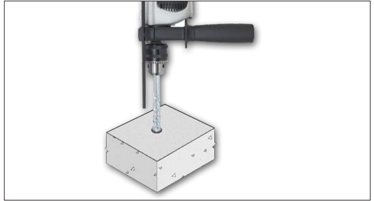
Figure D. Drill hole in concrete to accept the anchor bolt.
