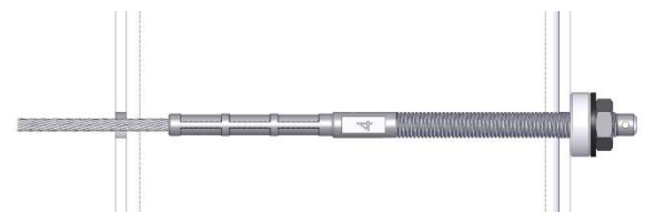
Figure E. Attach the first cable to the swage terminal. Place the plastic insert, washer and nut on the end of the shank and pull the cable tight.
