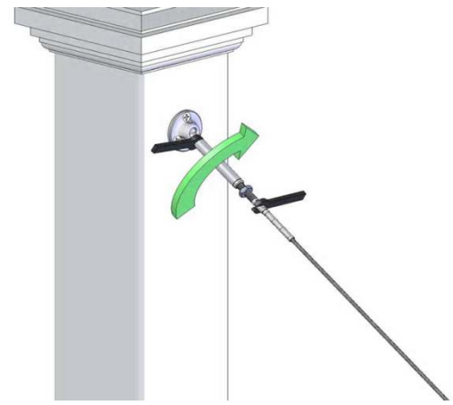
Figure R. Hold the swage terminal still with a 3/16" wrench and using a 5/16" open wrench, rotate tensioner body to tension.
