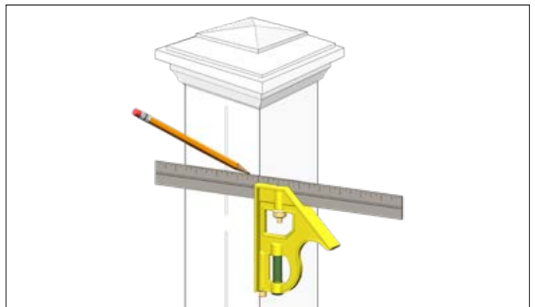
Figure C. Use a square and tape measure to mark the center of your posts.
