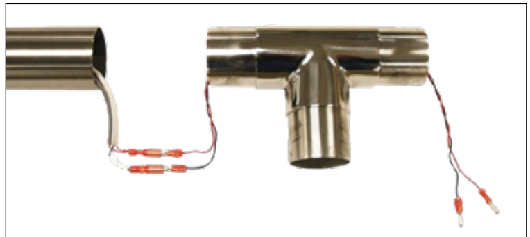
Figure C. Run supplied jumper wires between all fittings, including tees, elbows and 3-way corners. Adjustable fittings and dovetails should already have jumpers installed for your convenience.
