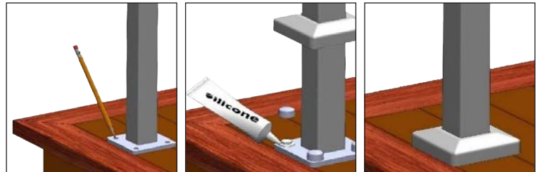
Figure C. (Left) Use the base as a template and mark the four (4) holes for the screws.
