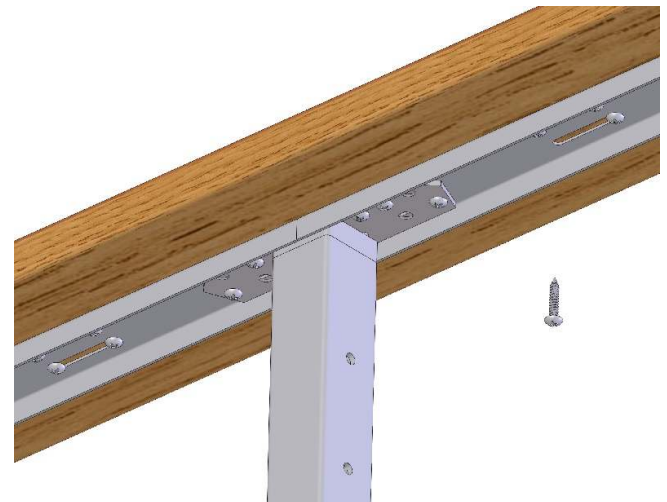
Figure AA. Use the supplied fasteners to attach the channel and top mounting plate to the top rail.
