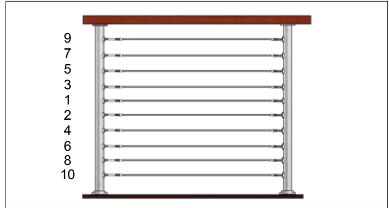
Figure H. Tensioning Diagram - Begin with the center run of cable and alternate working above and below until cables are tight.
