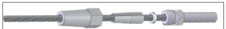
Figure F. Insert the cable into the receiver cone, wedge and spacer until it is fully seated in the threaded stud.
