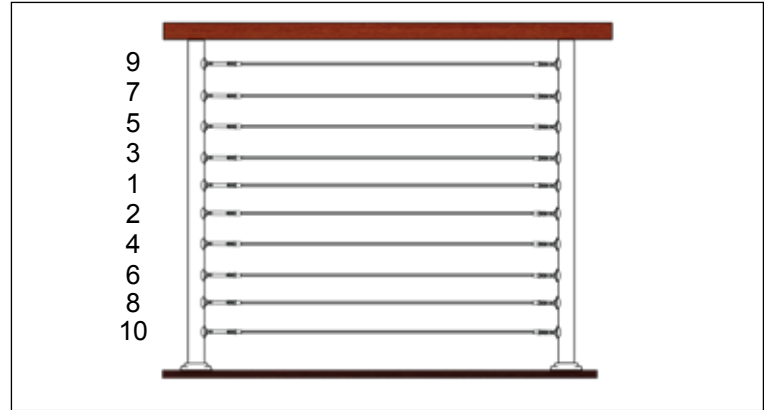
Figure H. Tensioning Diagram - Begin with the center run of cable and alternate working above and below until cables are tight.
