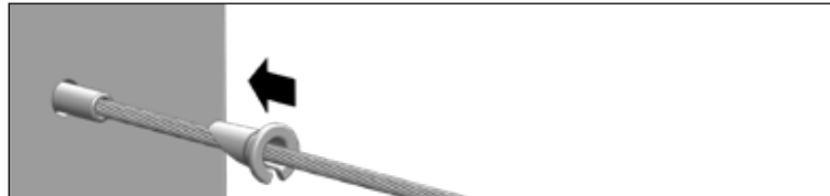
Figure BF. Push the tapered end onto the HandiSwage Stud and into the end or corner post hole.
