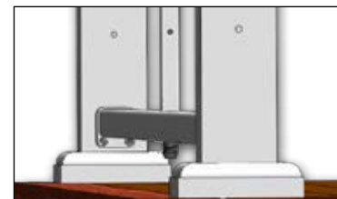
Figure M. (Left) Secure the bottom bracket with self-drilling screws.
