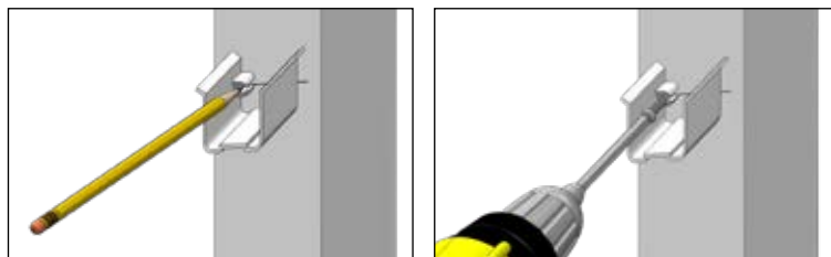
Figure AG. Mark the saddle bracket hole locations and attach with self-drilling screws.
