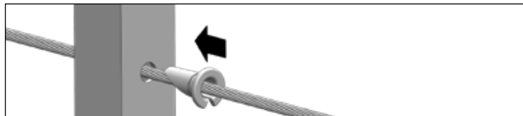
Figure BH. Push the tapered end into the mid post or cable stabilizer hole.
