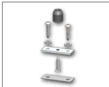
Figure K. (Left) Secure the bottom bracket with self-drilling screws.
