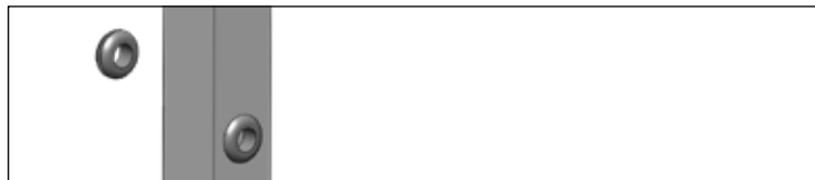
Figure BI. Affix the NOVA Stair Stabilizer Grommet around each hole in the stair stabilizer.
