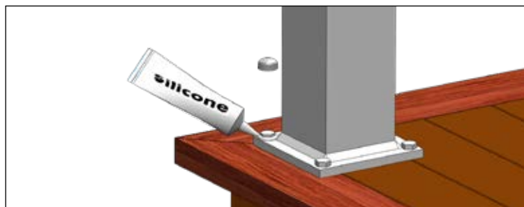
Figure C. Apply silicone to the top of the lag bolts and secure the lag bolt caps to prevent moisture from penetrating the holes.
