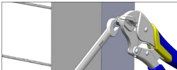
Figure U. Option one (1) is to hold the back of the stud with vice grips while tightening the nut.
