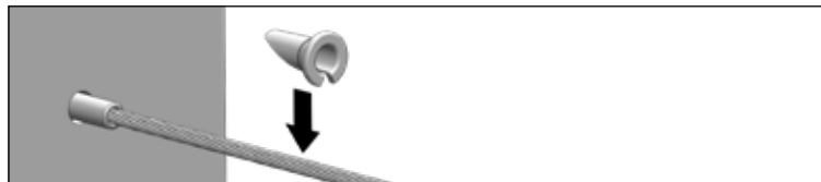
Figure BE. Place the slotted side on the cable and push down.
