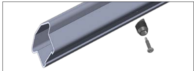
Figure AL. Install the stabilizer and support block connectors using a 1" self-drilling screw.
