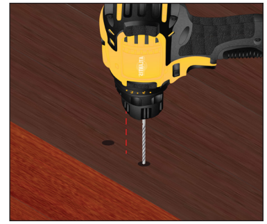
Figure U. (LEFT) Drill pilot holes at the pencil marks in the bottom side of the handrail.
