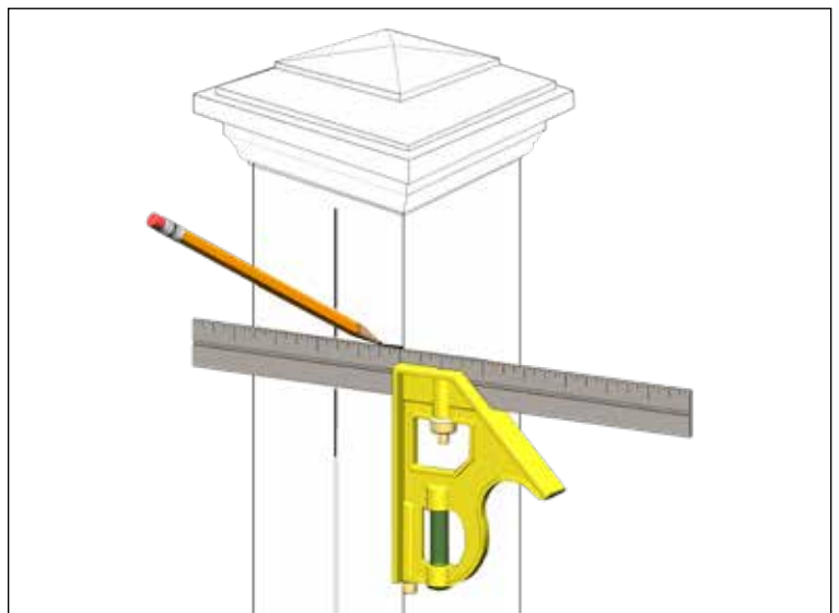
Figure A. Use a square and tape measure to mark the center of your posts.
