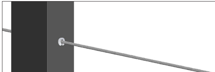
Figure W. The mid grommet helps prevent movement and deflection of the cable.
